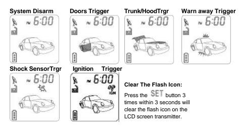
**TAMPER DISARMING**: If alarm triggered, upon disarm the system, siren chirp 4 times, parking light flash 3 times.
